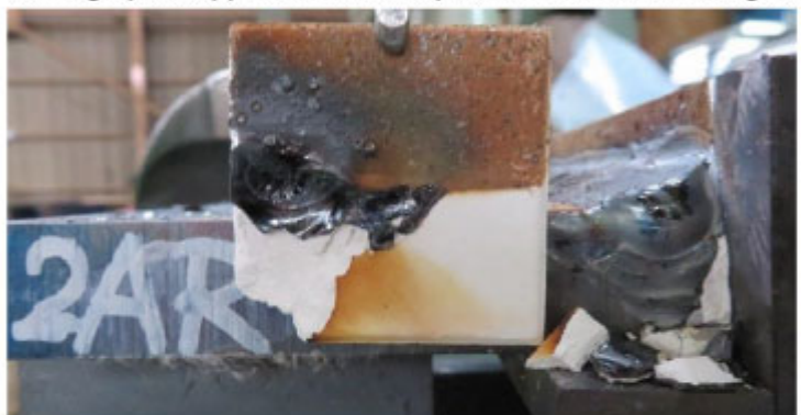
Photograph 7: Appearance of the specimen 2AR after welding (at the ending side)
