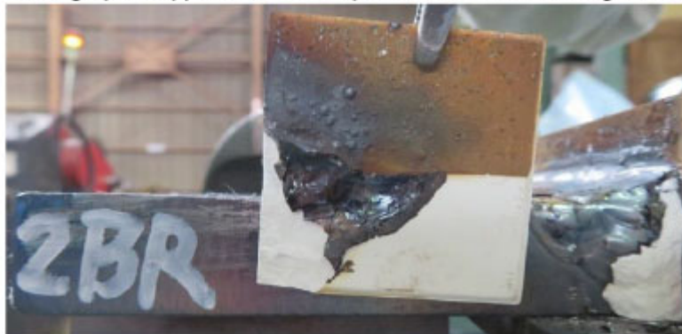
Photograph 9: Appearance of the specimen 2BR after welding (at the ending side)
