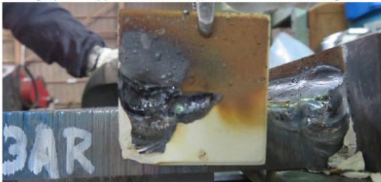
Photograph 11: Appearance of the specimen 3AR after welding (at the ending side)
