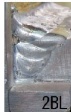
Photograph 8: Appearance of the specimen 2BL after welding (at the starting side)
