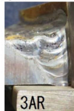
Photograph 11: Appearance of the specimen 3AR after welding (at the ending side)
