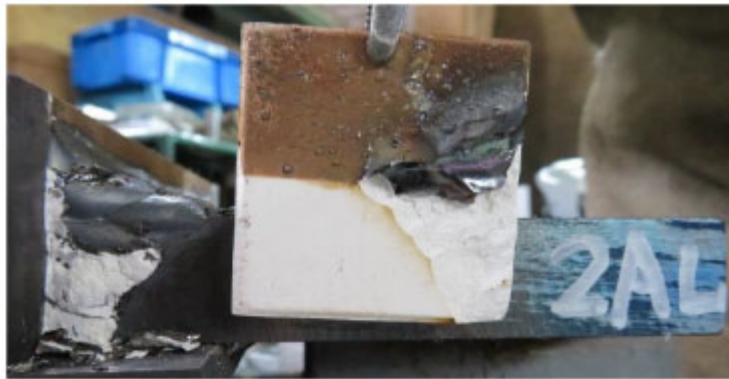
Photograph 6: Appearance of the specimen 2AL after welding (at the starting side)
