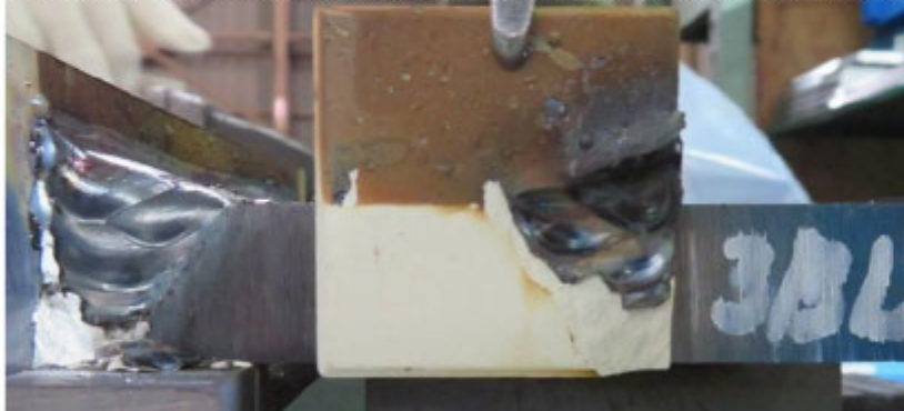
Photograph 12: Appearance of the specimen 3BL after welding (at the starting side)
