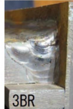
Photograph 13: Appearance of the specimen 3BR after welding (at the ending side)
