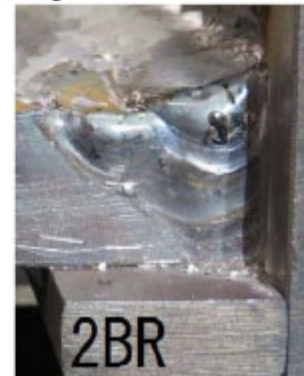
Photograph 9: Appearance of the specimen 2BR after welding (at the ending side)
