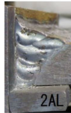
Photograph 6: Appearance of the specimen 2AL after welding (at the starting side)
