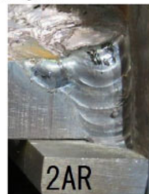
Photograph 7: Appearance of the specimen 2AR after welding (at the ending side)
