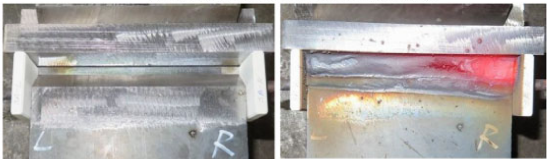
Photograph 4: Specimen 3A before and after welding
