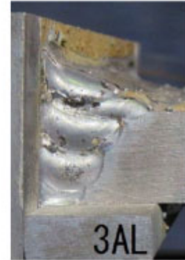
Photograph 10: Appearance of the specimen 3AL after welding (at the starting side)
