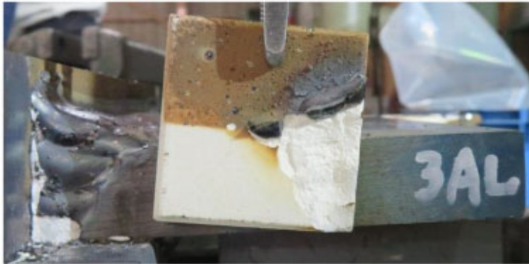
Photograph 10: Appearance of the specimen 3AL after welding (at the starting side)
