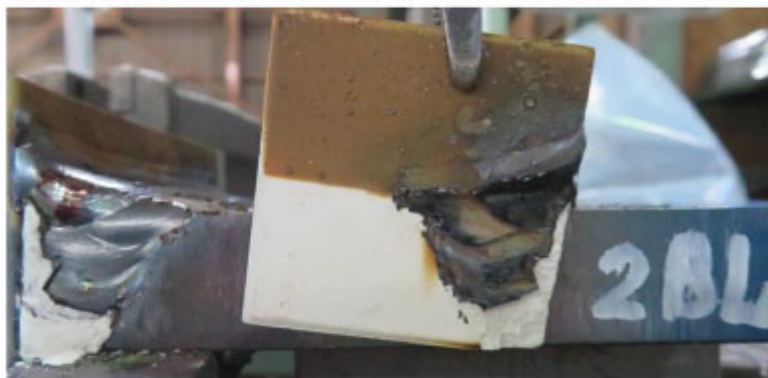
Photograph 8: Appearance of the specimen 2BL after welding (at the starting side)
