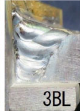
Photograph 12: Appearance of the specimen 3BL after welding (at the starting side)
